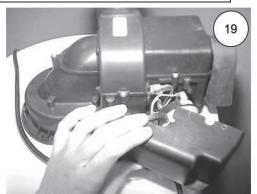
Remove three screws (Phillips Screw driver) from control access cover on blower and remove cover (see photo 19).
