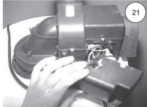
Remove three screws (Phillips screw driver) from control access cover on blower and remove cover (see photo 21).
