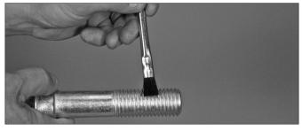
5. LUBRICATE BOLT THREADS: Apply a thin coat of Victaulic lubricant or silicone lubricant to the bolt threads. NOTE: If stainless steel bolts and nuts are special ordered, apply an anti-seize compound to the bolt threads.
