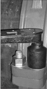
**7. TIGHTEN NUTS:** Tighten the nuts evenly by alternating sides (refer to the graphics on page 8 for the tightening sequence). Make sure the housings' keys engage the groove completely in each pipe end or AGS Vic-Ring. **Continue to tighten the nuts evenly by alternating sides until metal-to-metal bolt pad contact <b>AND** the **specified torque value are achieved.** Refer to the "Required Assembly Torques" table on the following page.
