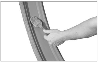
2. CHECK GASKET AND LUBRICATE: Check the gasket to make sure it is suitable for the intended service. The color code identifies the gasket grade. Apply a thin coat of Victaulic lubricant or silicone lubricant to the gasket lips, gasket exterior, and the interior surface of the coupling housings.
