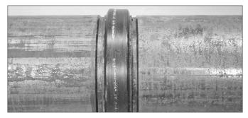
**4. JOIN PIPE ENDS:** Align and bring the two pipe ends together. Slide the gasket into position, and center it between the groove in each pipe end or AGS Vic-Ring.
