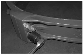
2. ASSEMBLE SEGMENTS: Assemble segments into two halves, as shown above. Install a flat washer (supplied with the coupling) onto the end of each bolt, and thread a nut finger-tight onto each bolt. NOTE: Make sure the oval neck of each bolt seats properly in the bolt hole. Tighten the nuts until metal-to-metal contact occurs at the bolt pads, then back the nut off a quarter turn.
