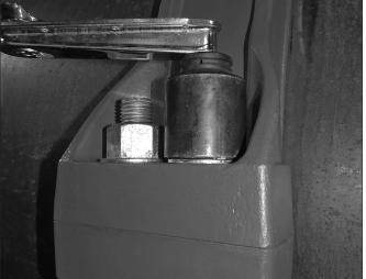
10. INSTALL BOLTS/FLAT WASHERS/NUTS: Insert the bolts. Install a washer onto the end of each bolt, and thread a nut onto each bolt finger-tight. NOTE: Make sure the oval neck of each bolt seats properly in the bolt hole.
