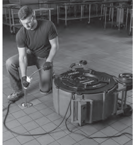
Figure 9 – Lubrification de la gaine de câble
