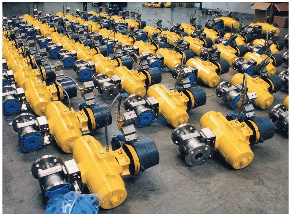
Automated packages with integral control actuation.
