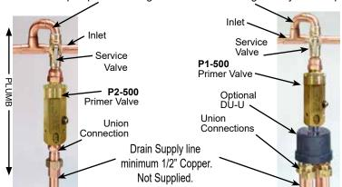
The Priming valve must have min. elevation of 12" (305mm) above the finished floor. Allow 1 foot of elevation for every 20 feet of distance run for floor drain make-up line.
