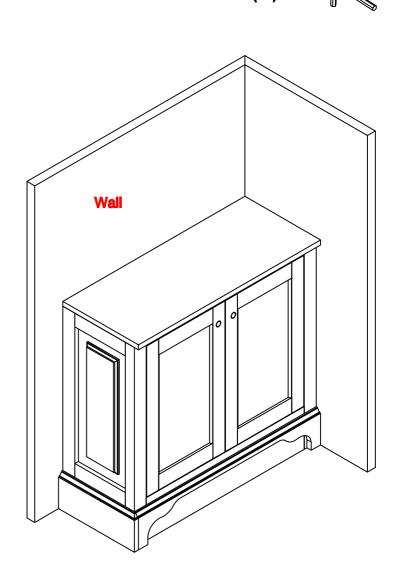
Note 1: De Soto cabinets feature removable side base moulding (Kick plates) to allow for flush placement against side walls and corners.
