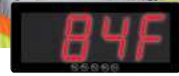
When the temperature reaches user specified setting, the display changes to red.
