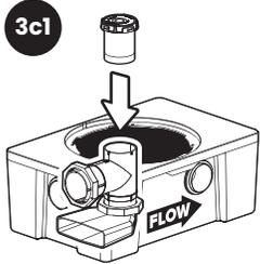
Slide flow control cartridge into top of inlet diffuser and rotate clockwise until cartridge drops onto flow control retainer pins. Continue rotating clockwise until pins are fully seated.
