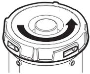
Rotate flow control cartridge counter-clockwise to release and remove from inlet diffuser
