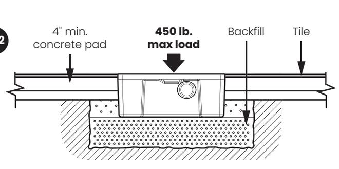
**Below Grade with Riser (preferred):** See instructions included with FCRI riser. Backfill evenly around tank using crushed aggregate (approximately 3/4" size rock or sand, with no fines), finish with a minimum 4" thick concrete pad.
