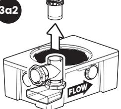
Rotate flow control cartridge counter-clockwise to release and remove from inlet diffuser
