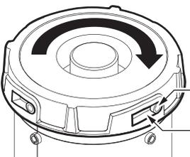
Slide flow control cartridge into top of inlet diffuser and rotate clockwise until cartridge drops onto flow control retainer pins. Continue rotating clockwise until pins are fully seated.
