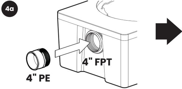
Choose inlet and outlet fittings (included) based on pipe size.
