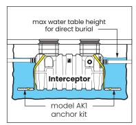
At risk areas include but are not limited to tidal surge areas, floodplains and areas that receive storm water. Great Basin™ models that are direct buried in high water table scenarios must be installed with an anchor kit. Model GB-500 uses model AKI anchor kit.
