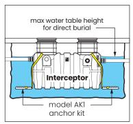
At risk areas include but are not limited to tidal surge areas, floodplains and areas that receive storm water. Great Basin™ models that are direct buried in high water table scenarios must be installed with an anchor kit. Model GB-500 uses model AKI anchor kit.
