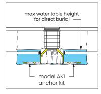
At risk areas include but are not limited to tidal surge areas, floodplains and areas that receive storm water. Great Basin™ models that are direct buried in high water table scenarios must be installed with an anchor kit. Model GB-50 uses model AKl anchor kit.
