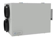
Suitable for very large residential or small commercial applications, the compact SER 260D comes with access panels on both sides of the unit for installation versatility. The SER 260D unit brings a continuous supply of fresh air into a home while exhausting an equal amount of contaminated air. The enthalpic core at the center of the unit transfers heat and moisture from the incoming air to the outgoing air that was cooled and dried by the building's air conditioner.
