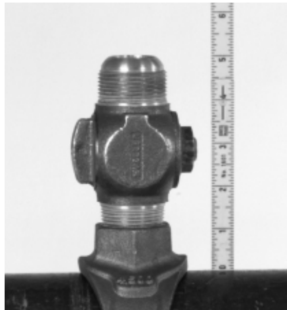
Figure 8 – Measuring valve standoff distance
