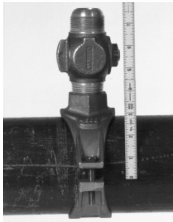
Figure 9 – Measuring valve standoff distance
