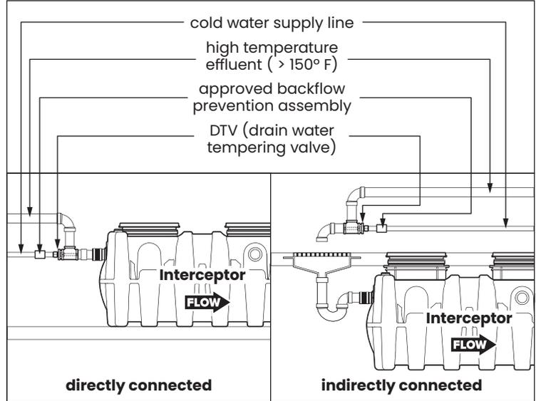
If water is entering the interceptor at excessive temperature (over 150° F), a drain water tempering valve (DTV) and approved backflow prevention assembly must be installed. Most state and local plumbing codes prohibit water above 150° F being discharged into the sanitary sewer. Water above 150° F will weaken or deform PVC Schedule 40 pipe, poly drainage fixtures like interceptors and erode the coating of cast iron (leading to eventual failure).
