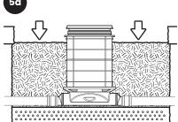
Backfill evenly around tank using crushed aggregate (approximately 3/4" size rock or sand with no fines) or flowable fill. **Do not compact backfill around unit.**
