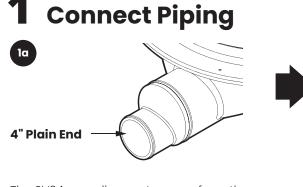
The SV24 sampling port comes from the factory ready to connect to 4" drain lines.
