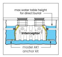
areas, floodplains and areas that receive storm water. Great Basin™ models that are direct buried in high water table scenarios must be installed with an anchor kit. Model GB-250 uses model AKI anchor kit.
