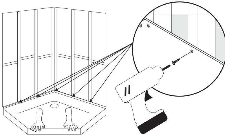
**3. Screw shower base flange to studs using 1/8' drill bit and flat head screws.**
