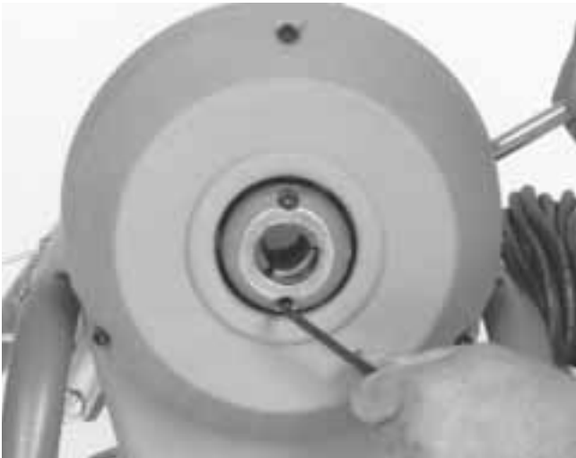
Figure 12 – Replacing Clutch Jaws
