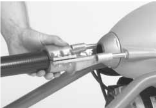
Figure 3 – Rear Guide Hose Attachment
