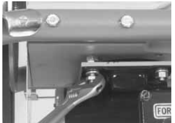
Figure 14 – Removing Clutch End Play
