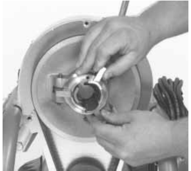
Figure 13 – Replacing Clutch Jaws
