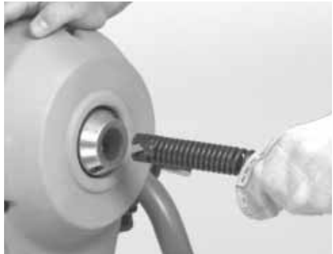
Figure 4 – Inserting Cable Into Front Of Machine
