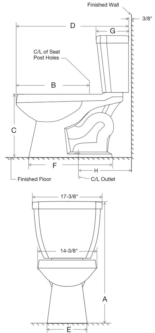
Note: All dimensions and specifications are nominal and may vary: Dimensions of 8" and greater have a tolerances of +3%. Dimensions less than 8" have a tolerances of +5%.
