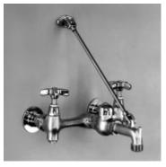
Chrome plated brass service sink faucet, 1/2" pipe eccentric inlets on 8" centers. Vacuum breaker integral stops, chrome plated (H&C) handles, 3/4" hose end spout with pail hook, top reinforcing bar and mounting bracket. Shall meet ANSI Specifications
