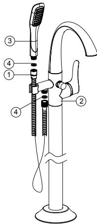
Connect one end of the shower hose (1) to the mixer (2) and the other end to the shower head (3). Ensure the washer (4) is into each end for seal.
