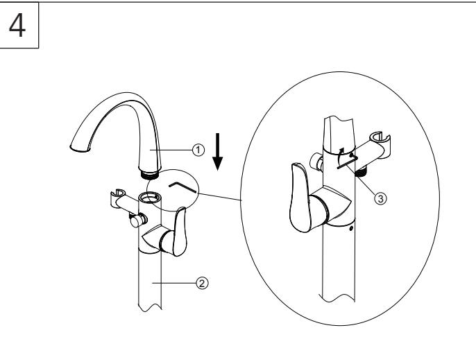
Insert the spout (1) into the faucet assembly (2) . Rotate the spout (1) to align correctly with the faucet assembly (2) then tighten the screw using hex wrench (3) (HEX:3.2mm).
