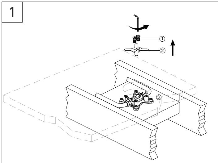
Shut off the water supply. Remove the old faucet. Clean the surface in preparation for the new faucet. Loosen the plug (1) with the hex wrench (HEX:6mm) and remove the guard plate (2) from the rough body (3).
