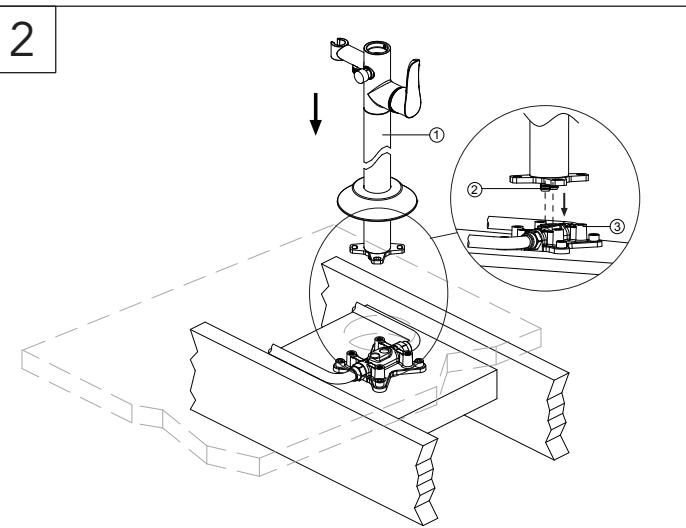
Locate the faucet assembly (1) onto the rough body (3), then push the connections (2) of inlet supply line into the rough body (3).
