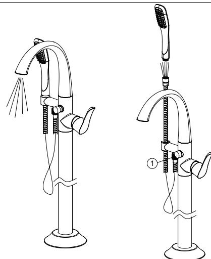
**IMPORTANT:** After installation is complete, turn on the hot and cold water supplies. Check for leaks. Flush the water lines for one minute. Press the pin (1) to the bottom position, and flush water lines for one minute. This flushes away any debris that could cause damage to internal parts. Check for leaks. After flushing, turn the handle all the way off to shut off the water. The pin should now be in its normal position. Re-tighten any connections if necessary, but do not overtighten.
