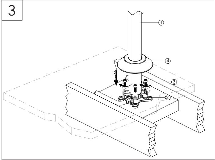
Secure the faucet assembly (1) to the rough body (2) using screws (3). Place the flange (4) over the standpipe and then push it to the base.
