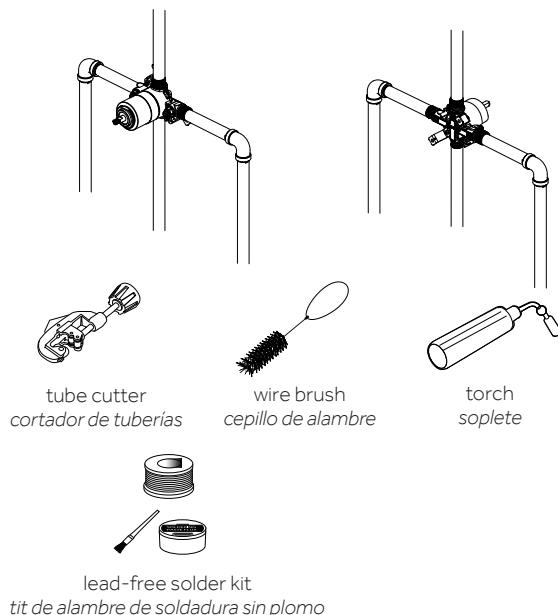
**Note:** Before soldering, remove the cartridge, stop valves and diverter cartridges.
