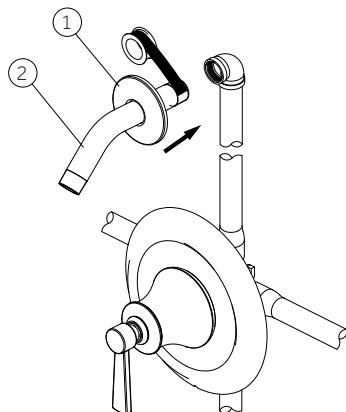
4. Install tub spout. Press tub spout onto pipe until spout is properly positioned and flush to the finished wall. Tighten screw (1) located at the bottom of spout with Allen wrench (Hex: 4.0mm).
