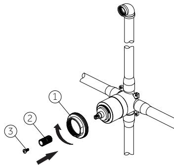
2. Position escutcheon (1) on valve body with drain hole (2) at the bottom. Place handle onto the brass stem extension and tighten handle seat (3).
