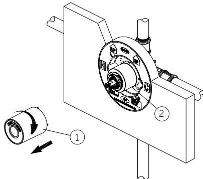
13. Rotate the lever counterclockwise until the water is to the maximum desired temperature, not to exceed 120 degrees F/49 degrees C. Seasonal maintenance of the maximum outlet temperature may be required due to changes in groundwater temperature.
