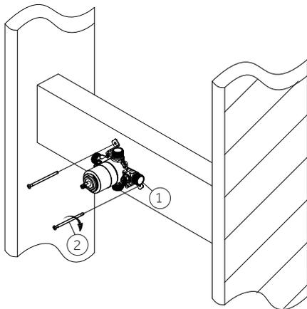
6. **With Tub Outlet:** Wrap plumbers' tape around the pipe threads in a clockwise direction. Connect the hot and cold water supply lines (1), the shower outlet pipe (2), and tub outlet pipe (3) by threading them onto the valve body (5) in a clockwise direction. Tighten the pipes to the valve body (5) with a pipe wrench. Connect the pipe elbows (4) to the end of the shower outlet and tub outlet pipes.
