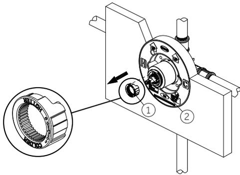
15. For colder water, adjust the limit stop ring (1) in a clockwise direction and reinstall the limit stop ring (1) onto the cartridge assembly (2). For hotter water, adjust the limit stop ring (1) in a counterclockwise direction and reinstall the limit stop ring (1) onto the cartridge assembly (2).
