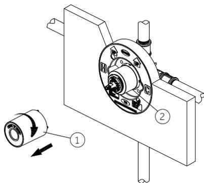
13. Rotate the lever counterclockwise until the water is to the maximum desired temperature, not to exceed 120 degrees F/49 degrees C. Seasonal maintenance of the maximum outlet temperature may be required due to changes in groundwater temperature.
