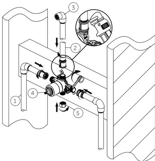
8. If the hot and cold inlets are reversed (hot on right and cold on left), remove bonnet (1) from the valve body (3) with reversed supply connections. Rotate the cartridge (2) 180°, so H appears on the right. Install the cartridge making sure that the key is fully engaged with the slot in the valve body (3). Slide the bonnet (1) over the cartridge (2) and thread them onto the valve body (3). Hand tighten securely.
