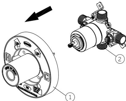
5. Fasten the body assembly (1) to cross brace with mounting screws (2).
