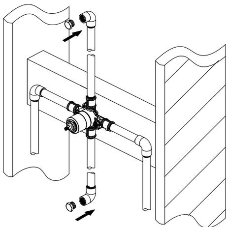
10. Turn on water allowing water to flow from tub outlet or shower outlet without tub spout until all foreign matter has cleared the line. Block one outlet using 1/2" iron pipe plug (1) to flush the debris out of the other outlet. Shut off water at faucet.
