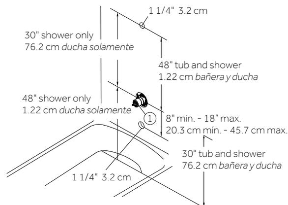
3a. **Thin Wall Installation:** Are usually built up with materials such as fiberglass tub surrounds and will be the main source of support for the valve. The plaster guard (1) remains attached to the valve.
