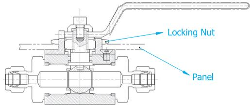
**Screw Hole for Panel Mounting**
