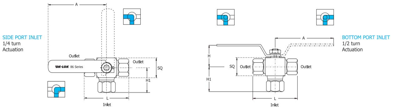
V86 3-way ball valve is designed to switch media through the inlet port and direct it to out of two outlet ports.
