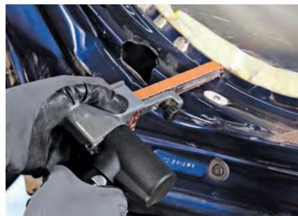
Using a belt rather than a drill bit is a quick, efficient and economical way to remove spot welded panels while leaving material to reattach the new or repaired panel.
