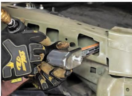
Grinding hard to reach spot welds, or even through a seized or stripped bolt is easy with Dynabrade belt tools that allow technicians to access tight areas with greater control.
