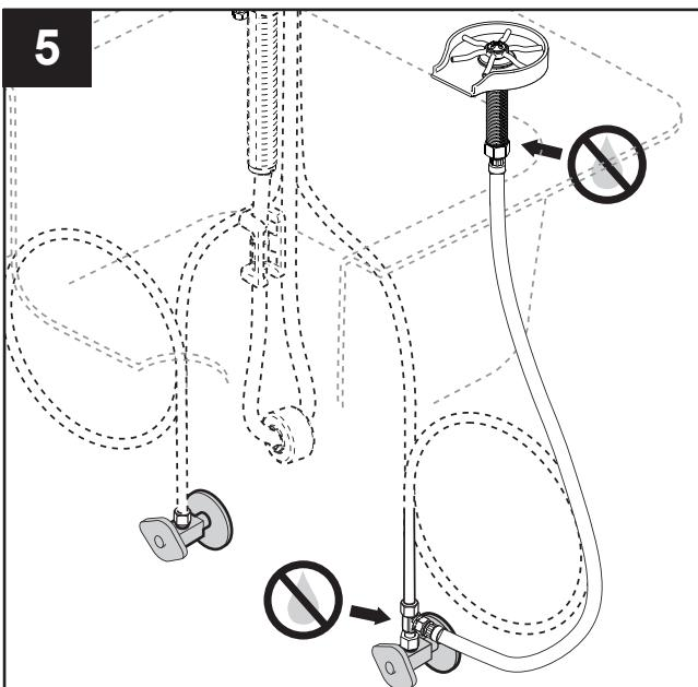
Turn on both water supplies at angle stops and check for leaks at all connections made during this installation.
