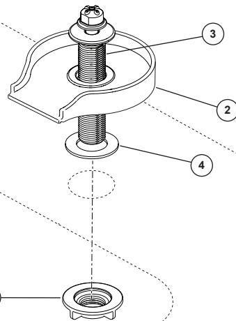
Slide mounting shank (3) through base (2) and steel support washer (4) from above. Support washer (4) if provided, sits on top of sink. Lower this assembly through sink from above. Ensure base is aligned with sink and outlet extends into basin prior to fully tightening mounting nut (5).
