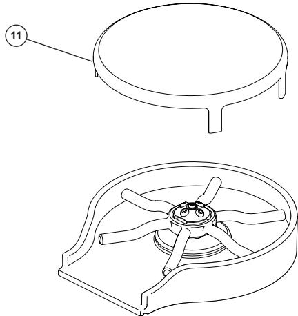
The cover (11) can be set in place for aesthetic purposes and to prevent unintended activation when the glass rinser is not in use. The front of the cover is marked on the underside of cover for best fit.
