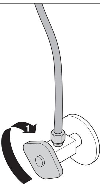
Turn off hot and cold water supplies at angle stops.
