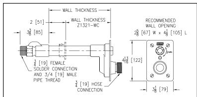
**ENGINEERING SPECIFICATION:** ZURN Z1321 Exposed Ecolotrol anti-siphon automatic draining wall hydrant. Complete with copper casing, all bronze interior parts with one-half turn ceramic disc cartridge and combination 3/4" [19 mm] female solder and 3/4" [19 mm] male pipe thread inlet. Stainless steel face with operating key. (All solder connections are lead free.)
