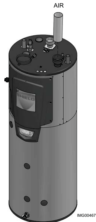
Figure 2-6 Near Water Heater Air Piping
