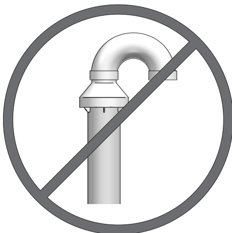
Figure 4-5 Do Not Install U-Bent to Rain Cap
