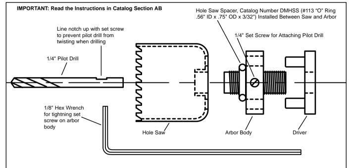
NOTE: Do Not Use Pilot Drill When Drilling PVC Pipe
