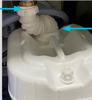
INSERT WASTE LINE INTO WASTE WATER TANK
