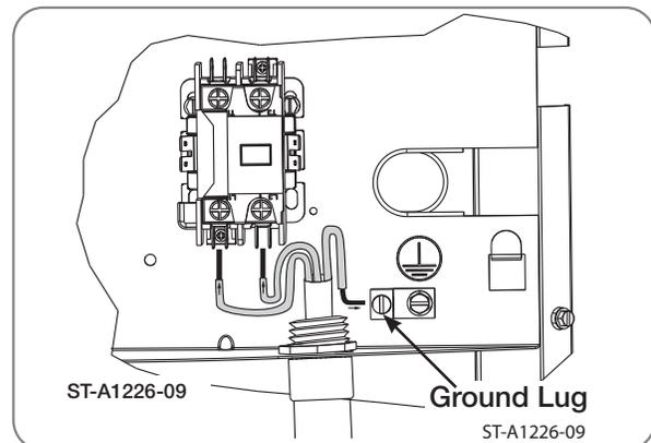
A grounding lug is provided near the line-voltage power entrance for a ground wire as shown in the above illustration.
