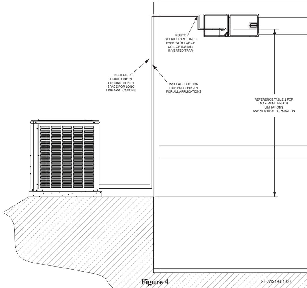
For applications that are considered to have a long line set with the outdoor unit below the indoor unit the following is required:
