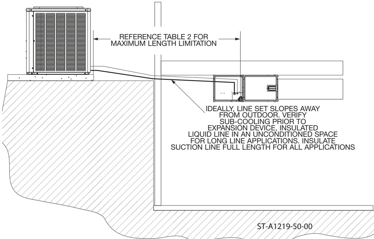
For applications that are considered to have a long line set with the outdoor unit and indoor unit near the same level the following is required:
