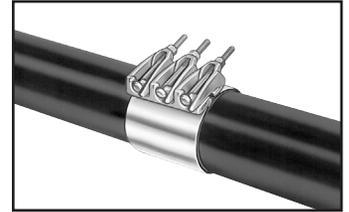
Squeeze the two lug sections together. Tighten the bolts evenly with incremental torque settings, up to the recommended torque.
