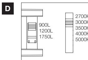
**STEP 4: Important!** The color temperature and light levels must be set on the fixture before installation into the ceiling. (Figure D)
