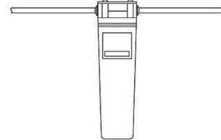
Pushing tube in before pulling it out helps to release tube
