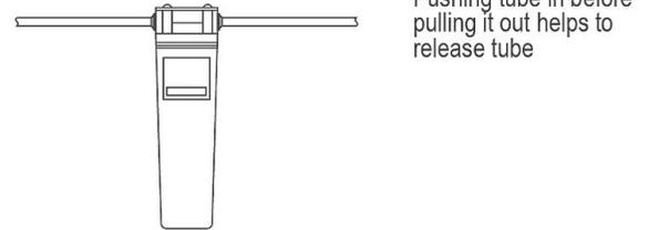
Pushing tube in before pulling it out helps to release tube
