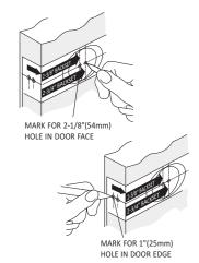
Fold Template below on Fold Line and Mark Door for Lock Bore Hole at 2-3/4" or 2-3/8" Backset and lock Edge Hole Centered on the door
