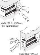
Fold Template below on Fold Line and Mark Door for Lock Bore Hole at 2-3/4" or 2-3/8" Backset and lock Edge Hole Centered on the door edge. Note: Most exterior doors
