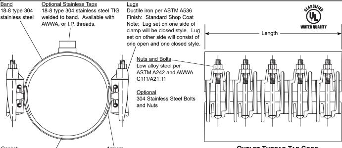
Gridded Virgin SBR compounded for water service, per ASTM D2000. NBR (Buna-N) is optional.
