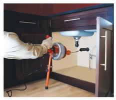
5. Slide the Grip Shield forward to release the Snake Grippers (or rotate the chuck to release the cable) and rock the machine back.
