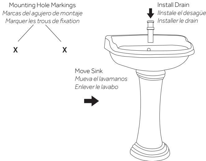
3. Drill pilot holes at the marked locations of the sink's mounting holes. If using anchors, insert the anchors into the drilled holes.
