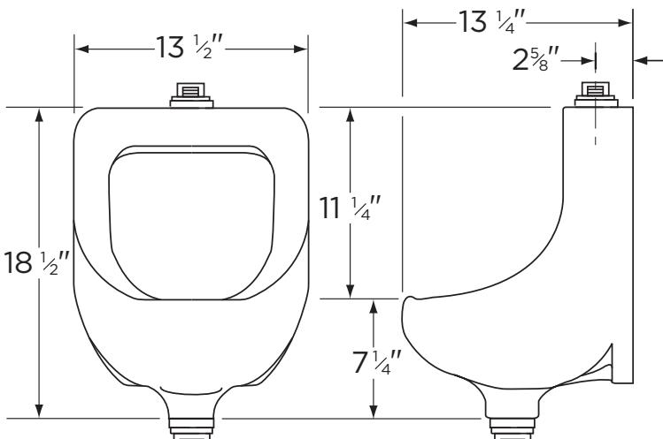
RECOMMENDED STATIC WATER PRESSURE FOR PLUMBING FIXTURES IS 20 - 80 PSI STATIC PER ANSI STANDARDS A112.19.2M APPENDIX B.
