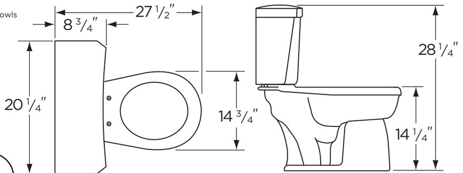
THIS FIXTURE QUALIFIES ACCORDING TO ASME TEST PROCEDURES AS A LOW CONSUMPTION WATER CLOSET WITH AN AVERAGE CONSUMPTION OF 1.6 GAL. OR LESS.
