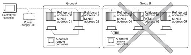
In group B, M-NET address of the outdoor unit whose refrigerant address is "00" is not set to the minimum in the group. As "03" is right for this situation, the setting is wrong. Taking group A as a good sample, set the minimum M-NET address in the group for the outdoor unit whose refrigerant address is "00".
