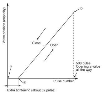
When the power is turned on, 700 pulse closing valve signal will be sent till it goes to @ point in order to define the valve position.
