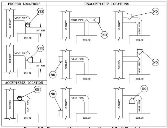
Figure 6-2: Proper and Improper Locations of Draft Regulator
