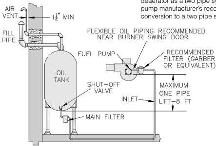
Figure 8-1: Single Pipe Oil Line
