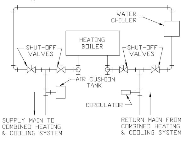
Figure 4-1: Recommended Piping for Combination Heating and Cooling (Refrigeration) System
