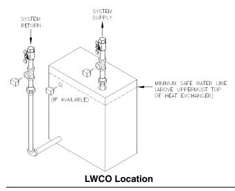
Select the appropriate size tee using the LWCO manufacturer's instructions. Often, the branch connection must have a **minimum** diameter to prevent bridging between the probe and the tee. Also, the run of the tee must have a minimum diameter to prevent the end of the probe from touching or being located too close to the inside wall of the run of the tee.
