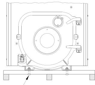
Figure 3-1: Packaged Boiler Removal from Skid
