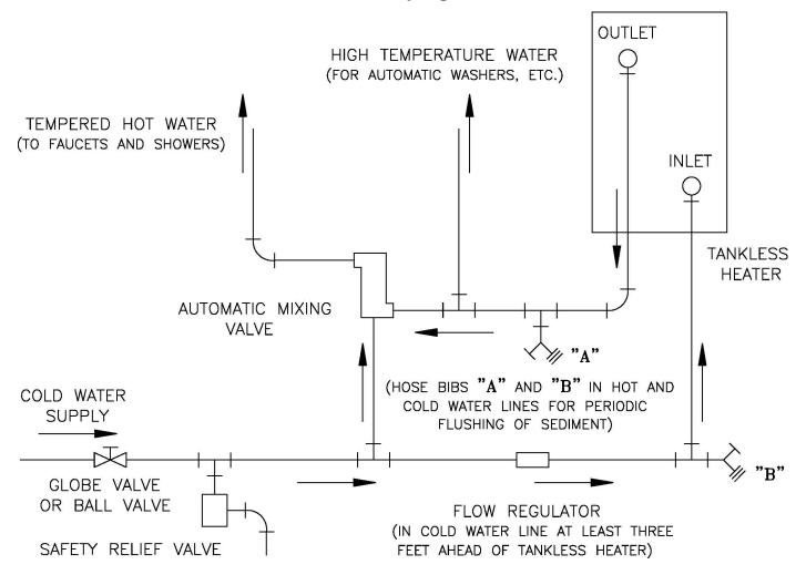
Figure 5-1: Schematic Tankless Heater Piping
