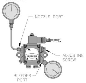
Figure 9-1: Adjusting Fuel Pump Pressure
