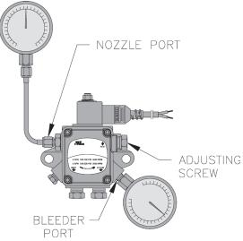
Figure 9-1: Adjusting Fuel Pump Pressure
