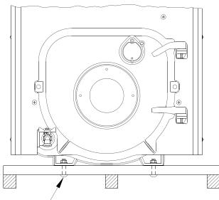
Figure 3-1: Packaged Boiler Removal from Skid
