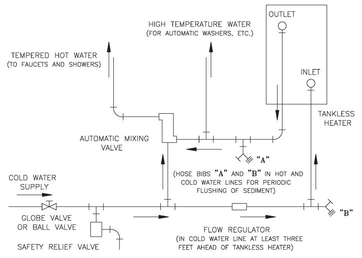
Figure 5-1: Schematic Tankless Heater Piping
