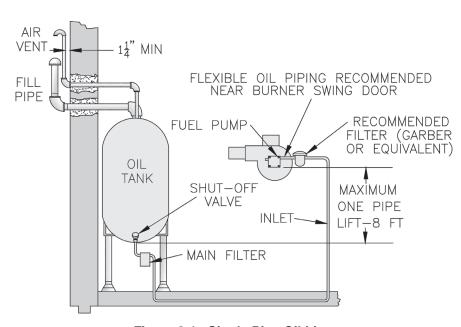
Figure 8-1: Single Pipe Oil Line
