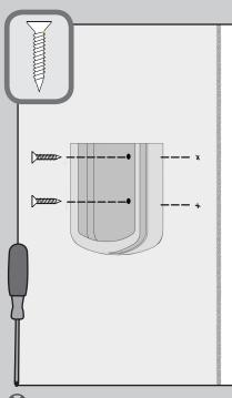
To install the transmitter cradle, hand-tighten the provided screws to mount the cradle to the wall.
