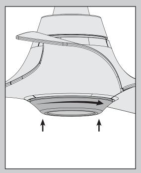
Carefully lift the glass lens cap up inside the LED assembly as far as it will go, then rotate the cap counterclockwise until it is held tightly in place by the tabs.
