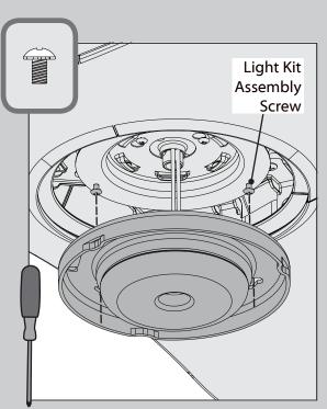
Screw two light kit assembly screws from the = hardware bag halfway into the upper switch housing. Push any excess wiring into the switch housing, then wrap the keyhole slots in the LED assembly around the screws and twist counterclockwise.
