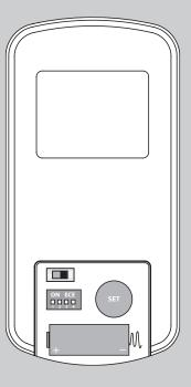
To change the battery, remove the battery door. Remove the battery and replace it with an A23 or MN21 alkaline battery.
