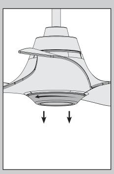
Carefully rotate the glass lens cap clockwise until it comes loose from the tabs and lower it from inside the LED assembly.
