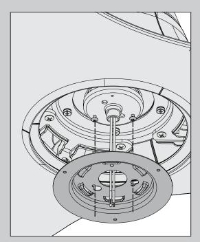
Feed the two single-pin connectors through the center hole of the upper switch housing, then wrap the keyhole slots around the screws and twist counterclockwise.
