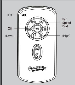
To select a fan speed press one of the numbers on the Fan Speed Dial. To calibrate the fan speed, run the fan on "6" for 90 seconds after each AC power reset. The LED light flashes to indicate a signal has been sent to the fan.
