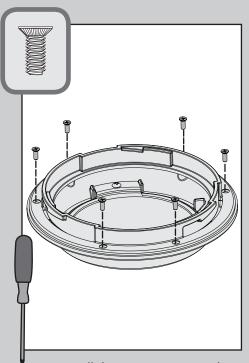
Uninstall the six screws around the outside of the glass lens cap. Remove the glass lens and set it aside for safe-keeping. Install the optional no-light cap using the same six screws. Tighten all six screws securely.
