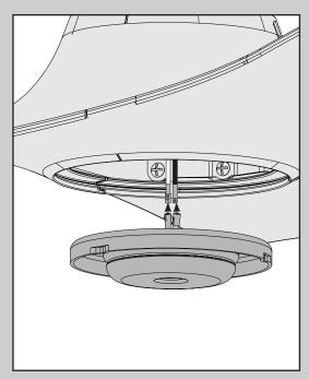
Connect the single-pin connectors from the LED assembly to the connectors from the fan.
