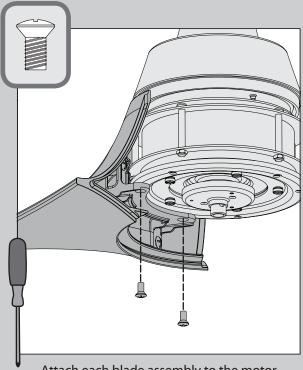
Attach each blade assembly to the motor housing as shown using two blade screws, found in the X hardware bag. Securely tighten the screws after all three blades are attached.
