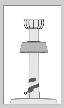
Slide the adapter cover onto the downrod, then hand tighten the downrod (at least 4-5 full turns) until it stops.
