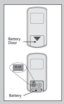
Remove the battery door. Change the DIP switch settings if the frequency matches a previously installed remote transmitter. Install an A23 or MN21 alkaline battery.
