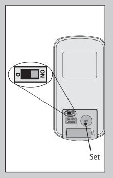
To pair the remote, hold down the Set button for 5 seconds. Pairing is complete when the LED button flashes twice. Move the toggle switch to "D" for full-range light dimming or "ON" for on/off function only.
