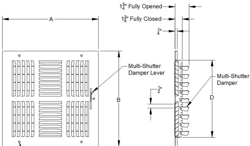
Countersunk Mounting Holes (6" x 6" and 8" x 8" will have 2 mounting holes, one on each side)
